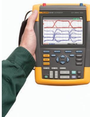
A handheld, battery-operated Fluke oscilloscope
