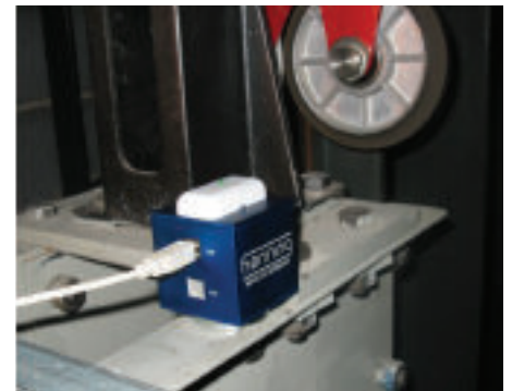
Figure 5: Accelerometer magnetically attached to crosshead
