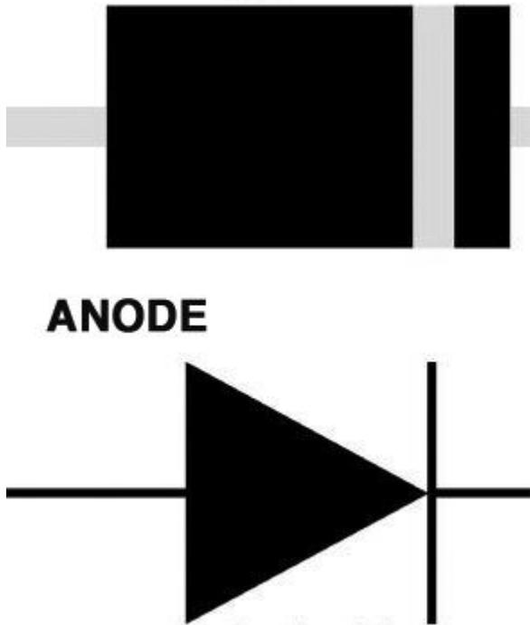
Pictorial (top) and schematic (bottom) of a diode: on the device, a single band denotes the cathode; on the schematic, an arrowhead is the anode.
