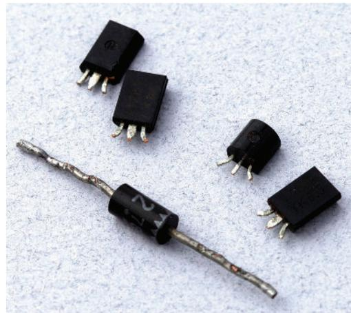
A diode with four transistors. Diodes usually have two leads and transistors have three leads. Sometimes a metal package is actually one of the terminals. Photo by Judith Howcroft
