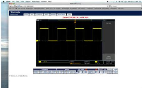
Prior to compensation, the square wave will have rounded corners or other distortion; after compensation, the square wave will not be deformed.
