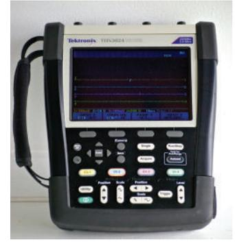
A handheld oscilloscope with all channels isolated from ground and isolated from one another
