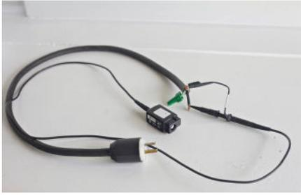
Power cord with a Tektronix TPP1000 probe connected
