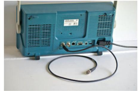
A BNC cable connected at the back panel of an oscilloscope
