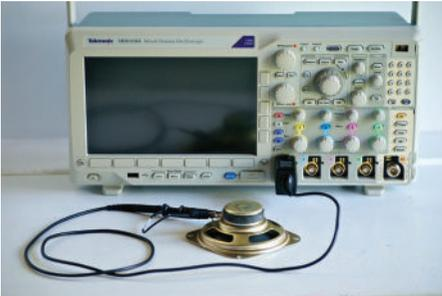
A probe connected to speaker removed from a discarded transistor radio: the polarity of the hookup does not matter, because the speaker is isolated from ground.
