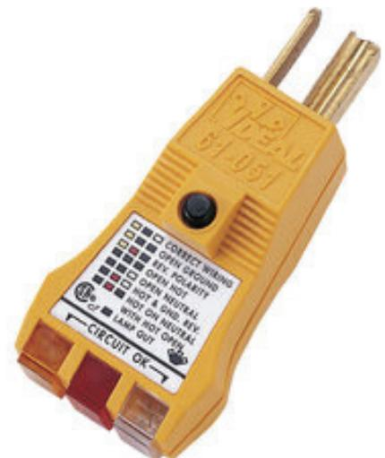
This inexpensive circuit analyzer will verify that the oscilloscope and equipment under investigation are connected correctly to the utility-supplied premises power.
