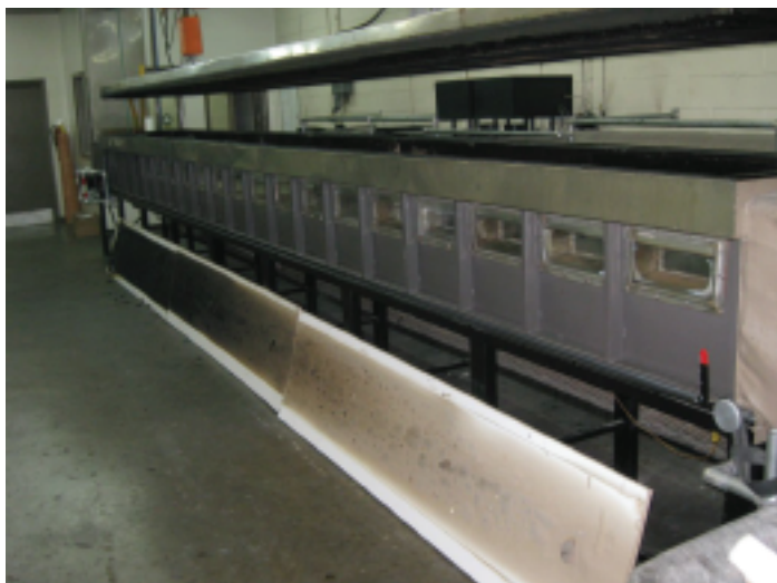
Figure 1: A Steiner Tunnel
