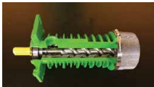
Figure 4: Section view of a submersible screw pump
