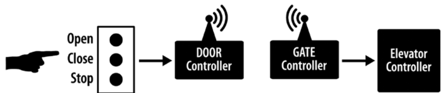
Figure 3: Landing door to elevator controller communication path
