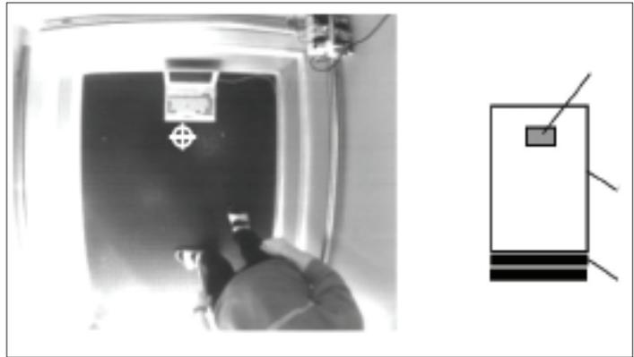
Figure 3: Incorrect mounting location for ESPROS/VOL-V in ceiling of elevator cab (0.5 m from back of elevator cab)
