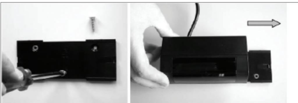
Figure 6: Fastening the mounting plate and then sliding the ESPROS housing on to the mounting plate
