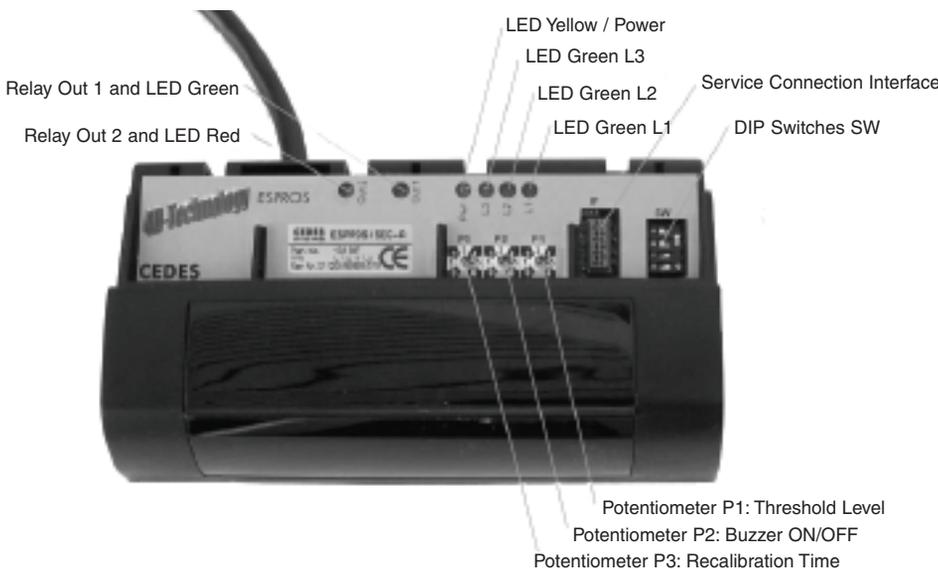
Figure 7: ESPROS/VOL indicators and configuration potentiometers/DIP switches
