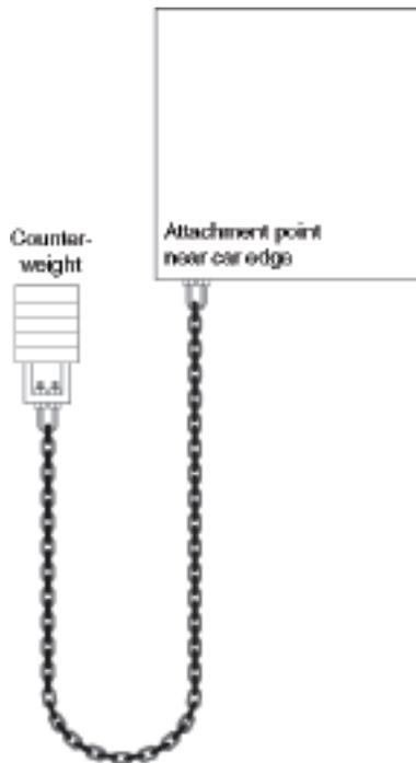
Compensation rope forms a loop as it hangs from its attachment points. The width of that loop depends on the flexibility of the compensation. Like the material it replaces, compensating cable forms a fairly narrow natural loop. Note that because of this narrow loop, the compensation is attached near the edge of the car.
