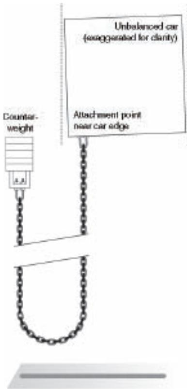
Elevator manufacturers determined that a hang length of approximately 400 feet (122 meters) for bare-chain compensation was about the maximum length for balance if the chain's support point was near the edge of the car. (Note: Maximum hang length for modern compensating cable is based on the strength of its support member and not the balance of the elevator.)
