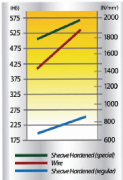
The Brinell hardness of your drive sheave is an important factor that needs to be considered when deciding upon the proper hoist rope.
