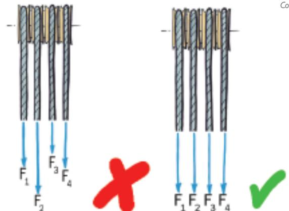
Failing to equalize hoist-rope tensions is one of the major causes of rope wear and overall system performance degradation.
