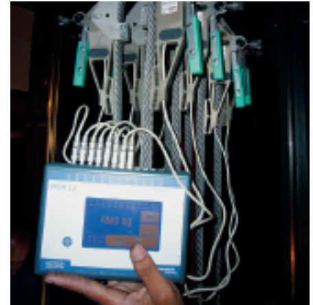
Figure 26: Rope Tensile Force measurement
