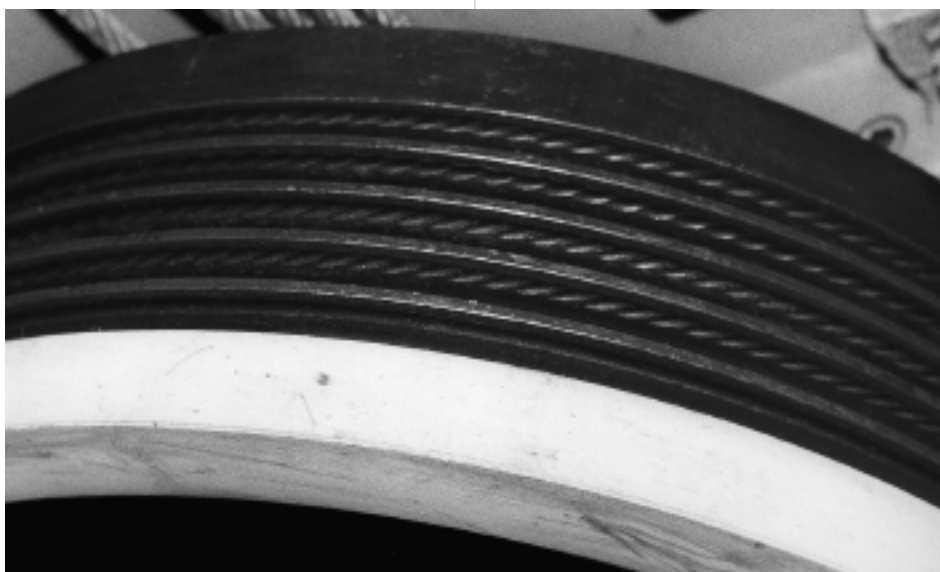
Figure 35: Rope impressions in the grooves of a traction sheave
