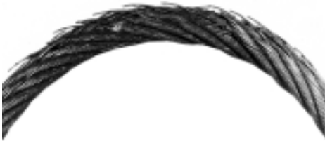
Figure 33: Inner wire breaks are visible when bent.
