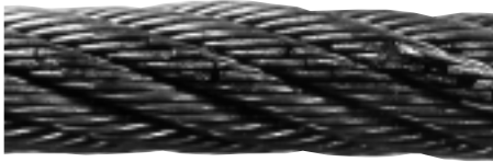
Figure 32: Inner wire breaks are visible when stretched.
